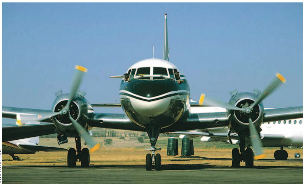
The Convairs are powered by two 3,000hp Pratt & Whitney R-2800-GB16 18-cylinder radials driving three-blade Hamilton Standard propellers.
